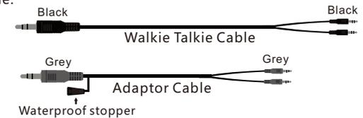
Packing includes walkie talkie cable with black plug, adaptor cable with grey plug (attached a black waterproof stopper). Please do not confuse the two different cables.
